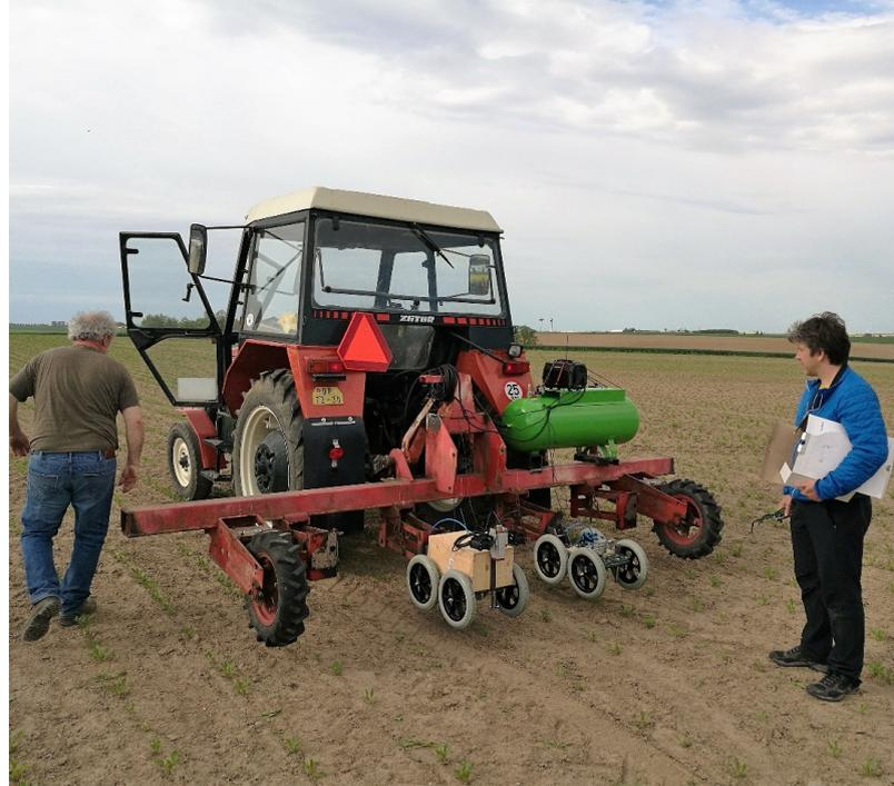
The weeding machine attached to a tractor.
