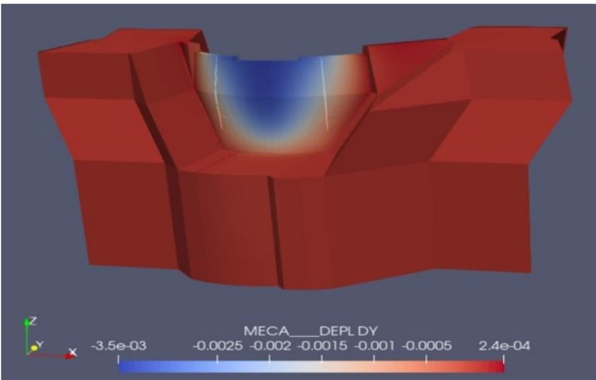
Figure 2: Results of modal deformation on a dam
