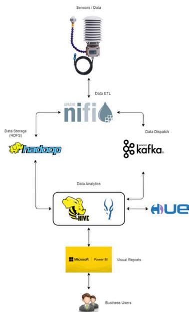
*Referential IoT Architecture for transferring and computational analysis of environmental (meteorological) data: Components and their communication links, within the realized referential IoT architecture.*
