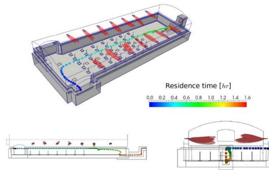
Figure 1. Tracing the glass particles inside the oven
