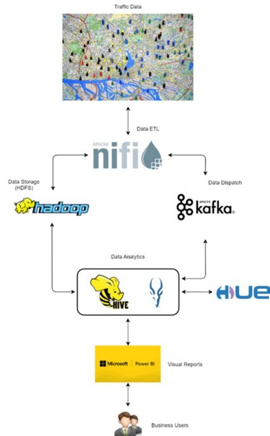
Referential IoT Architecture for transferring and computational analysis of traffic events data:
