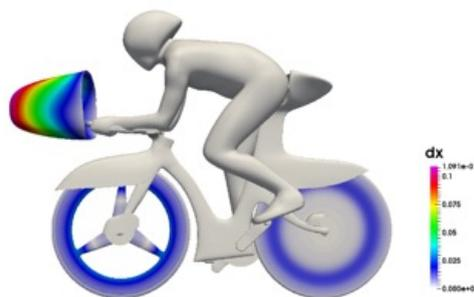
Figure 3: Change (in meters) in the various parts of the bicycle
