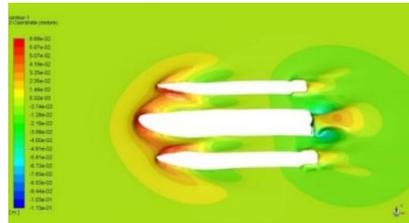
CFD simulation of the interactions between the trimaran hulls
