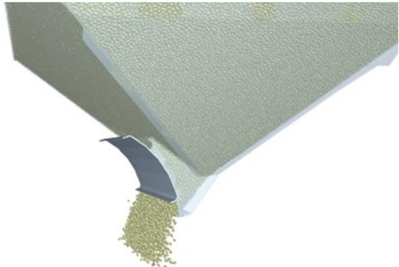
*Calculations of the frictional and normal force from the flowing bulk material (grain) on the hopper closing mechanism.*
